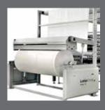
Magazine winder is recommended for winding heavy GSM tubular fabrics used for FIBC applications in which desired fabric tension can be adjusted by regulating torque through winder motor. The fabric roll is located above the ground level for ease of unloading with a forklift.
